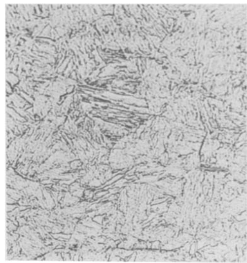
Figure 9 Microstructure of post-weld heat treated low-alloy steel, far from weld interface, etched in nital. Ferrite with little bainite and dispersed carbides (500 ×). HV_{10} = 206 .
